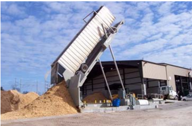
A load of wood chips is unloaded at the Intrinergy-owned boilerhouse location at the Coastal Paper site in Wiggins
